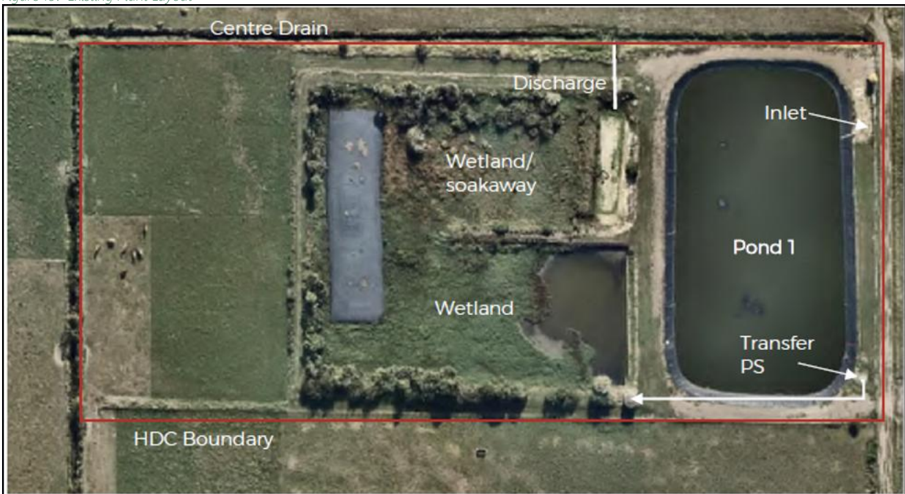
Figure 19: Existing Plant Layout
